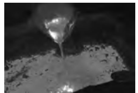
MOLTEN BRASS IN THE FURNACE
