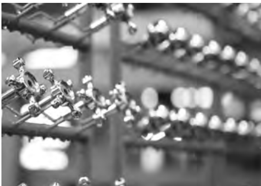
CROSTOP HANDLE BOSSES ARE RACKED AND PLATED IN-HOUSE
