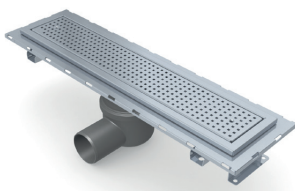
Central outlet with no falls built in for a shallower channel depth. Shown here with a stainless steel Chess grate
