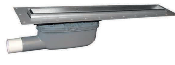
Side side/inline outlet Flow rate: min. 60 litres/minute Total channel height: 140-144mm
