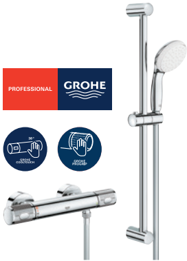
120140 £236.62 Grohtherm 1000 Performance thermostatic shower mixer set For low pressure systems Tempesta 100 2 spray shower GROHE Turbostat cartridge for reverse water ways GROHE ProGrip ergonomic handles have a knurled surface for great grip GROHE CoolTouch prevents scalding on hot surfaces
